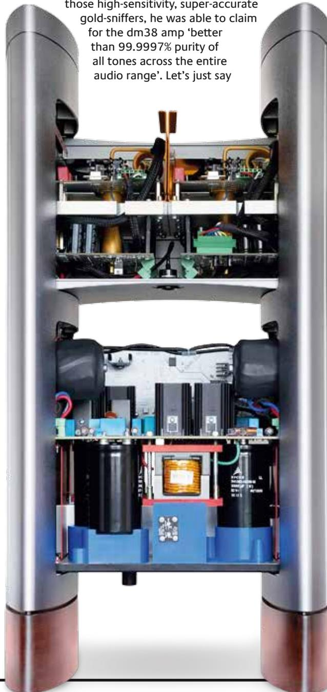
**RIGHT:** Inside, seen from the front, showing the dual switchmode PSU [lower enclosure] and modular, dual mono FET power amplifier [top enclosure]. The tall alloy limbs also form part of the efficient heatsinking
