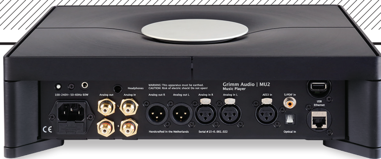
ABOVE: The MU2 offers a network control/streaming input, coax/optical S/PDIF and AES inputs, plus USB-A for external drives. Analogue line inputs and outputs are provided on both single-ended RCAs and balanced XLRs
